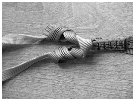
Figure 9 - pulled tight, it's a Prusik mess
