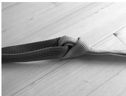
Figure 2 - one sling "girth hitched" to the other
